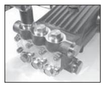
1. With a 30mm wrench, remove the six (6) plugs (48) from the valve casing (43). Inspect the o-rings (48A) and replace if necessary. Remove the complete valve assembly (46A) by threading a 12mm bolt into the spring retainer and pulling straight out.
